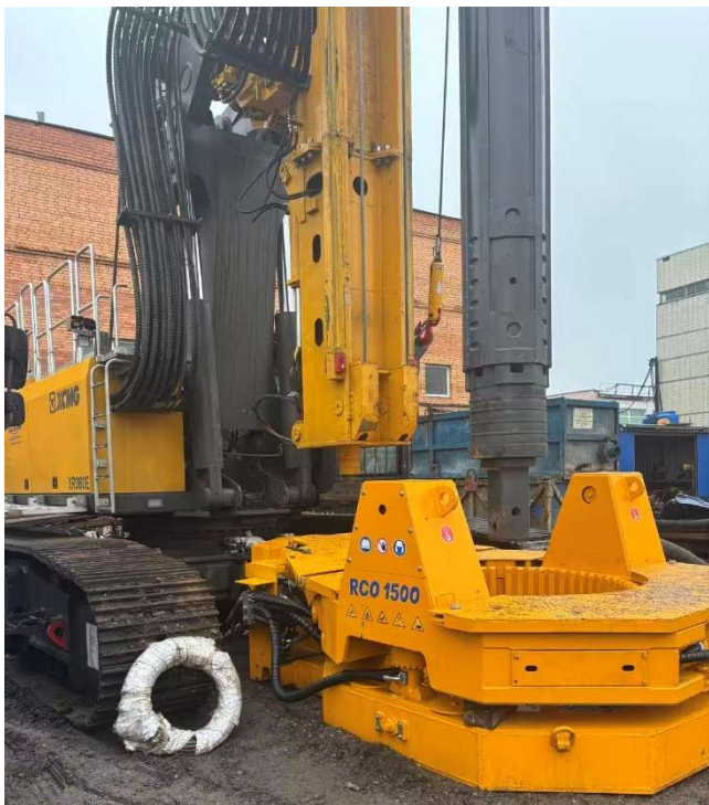
RCO 1500 with XCMG Drilling rig
