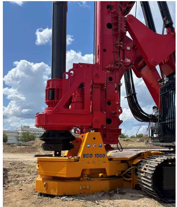
RCO 1500 with SANY Drilling rig
